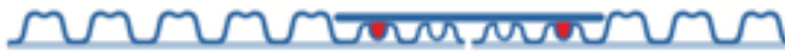
Pipes can be cut and corrugations reshaped to produce any length of pipe, in increments of one corrugation.
